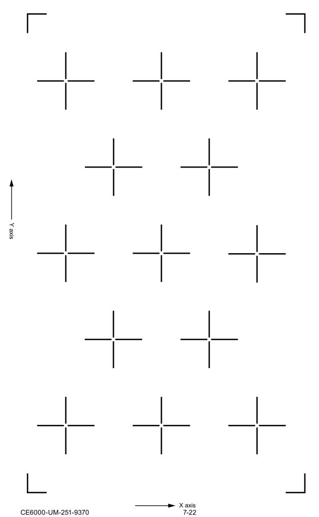
The specification of the cross mark is 30mm line length, and 0.3 to 0.5mm line width.
