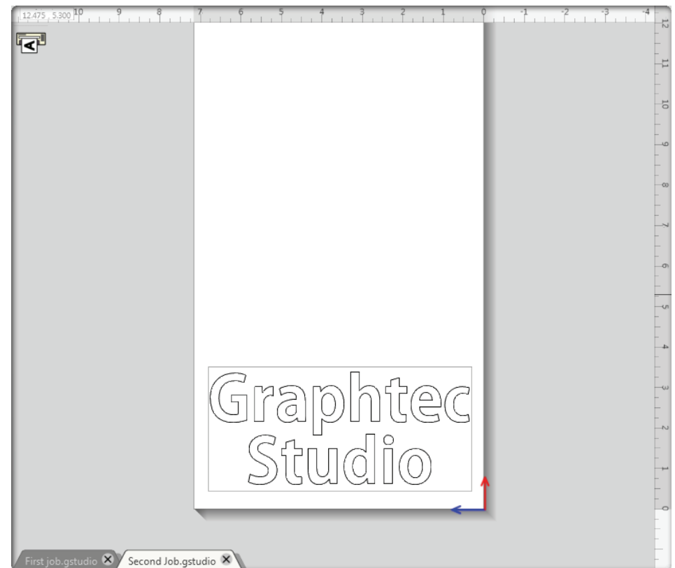
Here is the same design in the Output Mode of the Preview Area. Notice that it is given an outline showing how it is to be cut.
