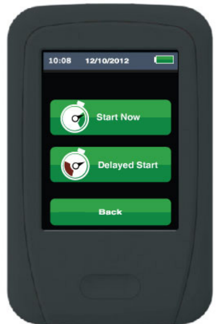
6. Choose to start logging immediately or to schedule a data logging session.
